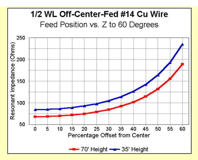
The third graph decompresses the second by cutting off the steepest part of the curve. It reveals the quite different feedpoint impedances for the two antennas as the feedpoint moves away from center.
