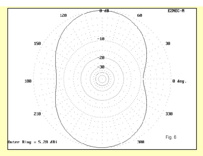
Figure 6 shows the azimuth pattern of our 7.15 MHz OCF with 35' of 300-ohm parallel feedline. With this length of radiating parallel feedline, the gain of the maximum lobes drops to about 5.9 dBi. The lost gain goes into the radiation off the ends, which is increased a few dB on each side of the pattern. The overall performance in this mode is essentially that of a basic dipole.
