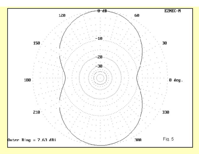
This pattern is taken from the 300-ohm feedpoint position, which (at this height) indicates a length of 10.4' on the short side of the feedloint and 57.35' on the long side. In this configuration, the asymmetry is barely noticeable, as the angle of maximum radiation bends by a mere 2 degrees from that of a dipole and the long end of the antenna shows about 2 dBi less indentation than the short side.
