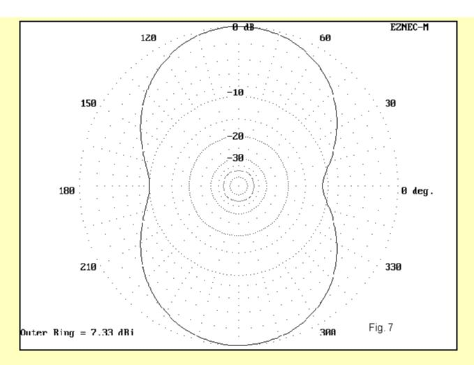
Figure 7 shows the azimuth pattern of an antenna meeting our assumptions. The gain of the main lobes is up to 7.3 dBi, but the radiation off the ends is down compared to the radiating parallel feedline. However, the differential among all three of our antennas is operationally insignificant.
