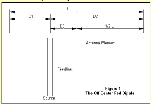
OCFs are derived from the Windom antenna, a 1929 concoction using a single- wire feed attached to the antenna element at what was believed to be the 600-ohm point. The single wire feedline was presumed to have an impedance of 600 ohms against ground.
