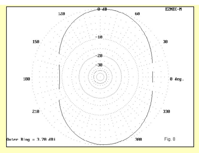
Figure 8 shows what happens if we increase the radiating parallel feedline to a full half wavelength. The gain drops to about 3.7 dBi, with a take- off angle of 24 degrees. The pattern is a significant oval (instead of a peanut): it yields a somewhat stronger signal off the ends--but no more than for an inverted Vee of moderate slope at the same peak height.
