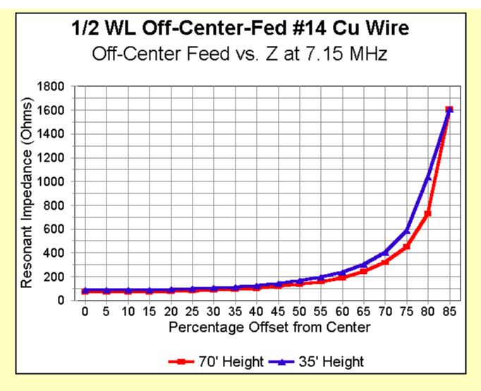
The second graph gives an overview of what happens to the feedpoint impedance of the antenna as that point is moved outward from center. Note that as the impedance passes through 300 ohms, the curve grows steeper rapidly, making the process of setting a 300-ohm feedpoint tricky at best. It is much easier to hit the 100-ohm feedpoint, but not quite as easy as this compressed graph suggests.
